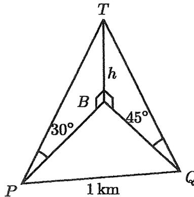
The angle of elevation from a boat at  $P$  to a point  $T$  at the top of a vertical cliff is measured to be  $30^\circ$ . The boat sails 1 km to a second point  $Q$ , from which the angle of elevation to  $T$  is measured to be  $45^\circ$ . Let  $B$  be the point at the base of the cliff directly below  $T$  and let  $h = BT$  be the height of the cliff in metres. The bearings of  $B$  from  $P$  and  $Q$  are  $50^\circ$  and  $310^\circ$  respectively.
